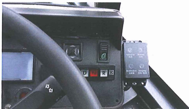
Telematics system provides visual cues to bus drivers when speeding, braking, accelerating or when driving abruptly, to encourage safer and more sustainable driving for an enhanced commuter experience.
